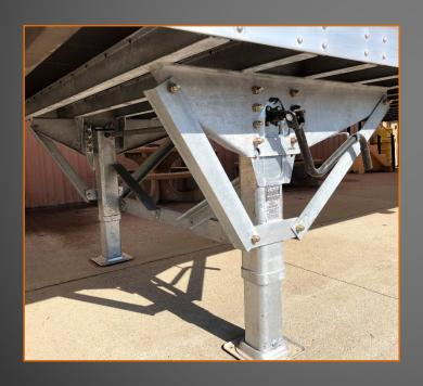
Next lower the landing gear enough to take the weight and pressure from the fifth wheel slider mechanism.
