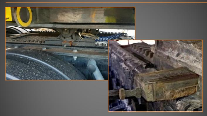
Next visually inspect the pins and ensure they are in the open (unlocked) position. The pins should be protruding out the side of the base allowing the fifth wheel to slide on the track.
