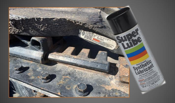
Spraying the slider tracks and the locking pins with a spray lube or apply some grease will help the device unlock and slide easier.
