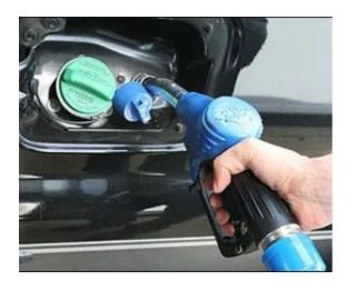
It is imperative a driver maintain adequate DEF on the truck to ensure regeneration. DEF consumption is approximately 1 gallon of DEF for every 50 gallons of fuel burned. If the truck runs out of DEF, the power will be reduced, and the speed may be limited to 5 mph until the DEF tank is refilled.
